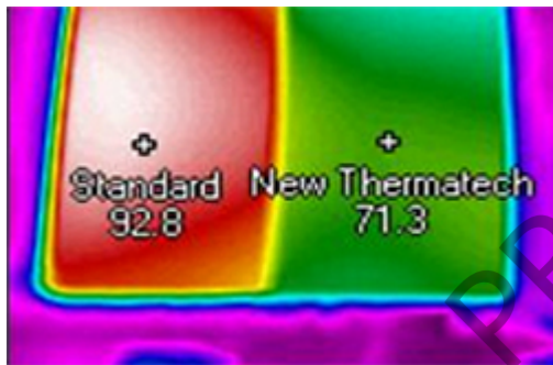
Next Generation COLORBOND® Ultra™ steel Readings in Degrees Celsius
